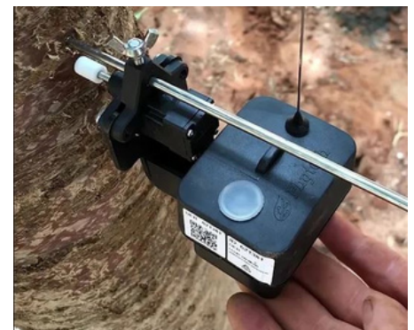
Trunk dendrometer to measure expansion and contraction
