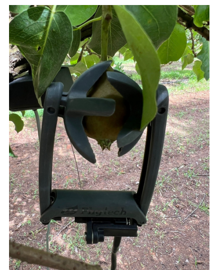
Fruit sensor to measure size
